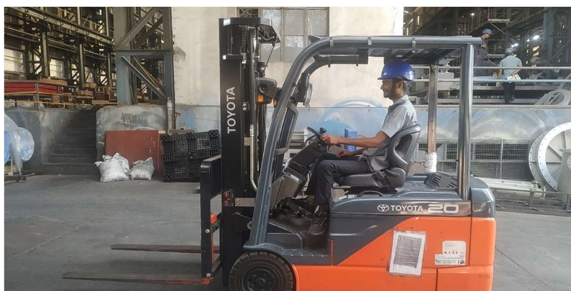
Fig. Battery operated forklift
